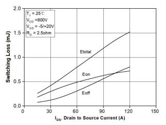
Figure 23. Clamped Inductive Switching Energy vs. Drain Current (V<sub>DD</sub> = 600V)
