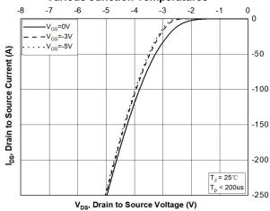
Figure 9. Body Diode Characteristic at T<sub>J</sub> = 25 °C
