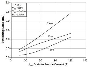
Figure 24. Clamped Inductive Switching Energy vs. Drain Current (V<sub>DD</sub> = 800V)
