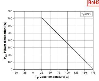
Figure 20. Maximum Power Dissipation Derating vs. Case Temperature
