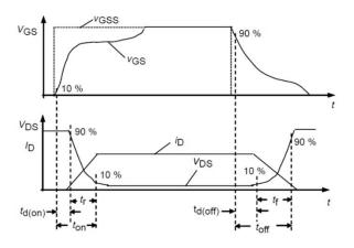
Figure 28. Switching Times Definition
