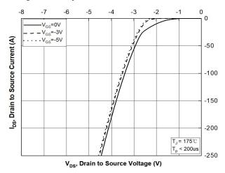
Figure 10. Body Diode Characteristic at  $T_J$  = 175 °C
