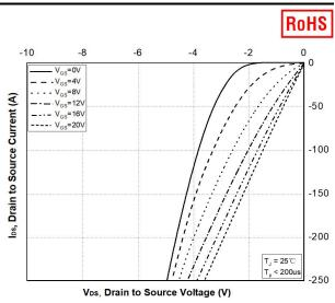
Figure 14. 3rd Quadrant Characteristic at T<sub>J</sub> = 25 °C
