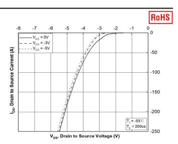
Figure 8. Body Diode Characteristic at T<sub>J</sub> = -55 °C
