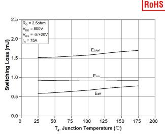
Figure 26. Clamped Inductive Switching Energy vs. Temperature
