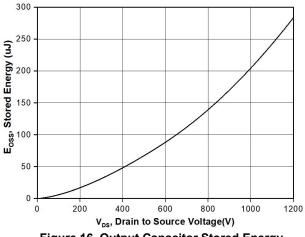
Figure 16. Output Capacitor Stored Energy
